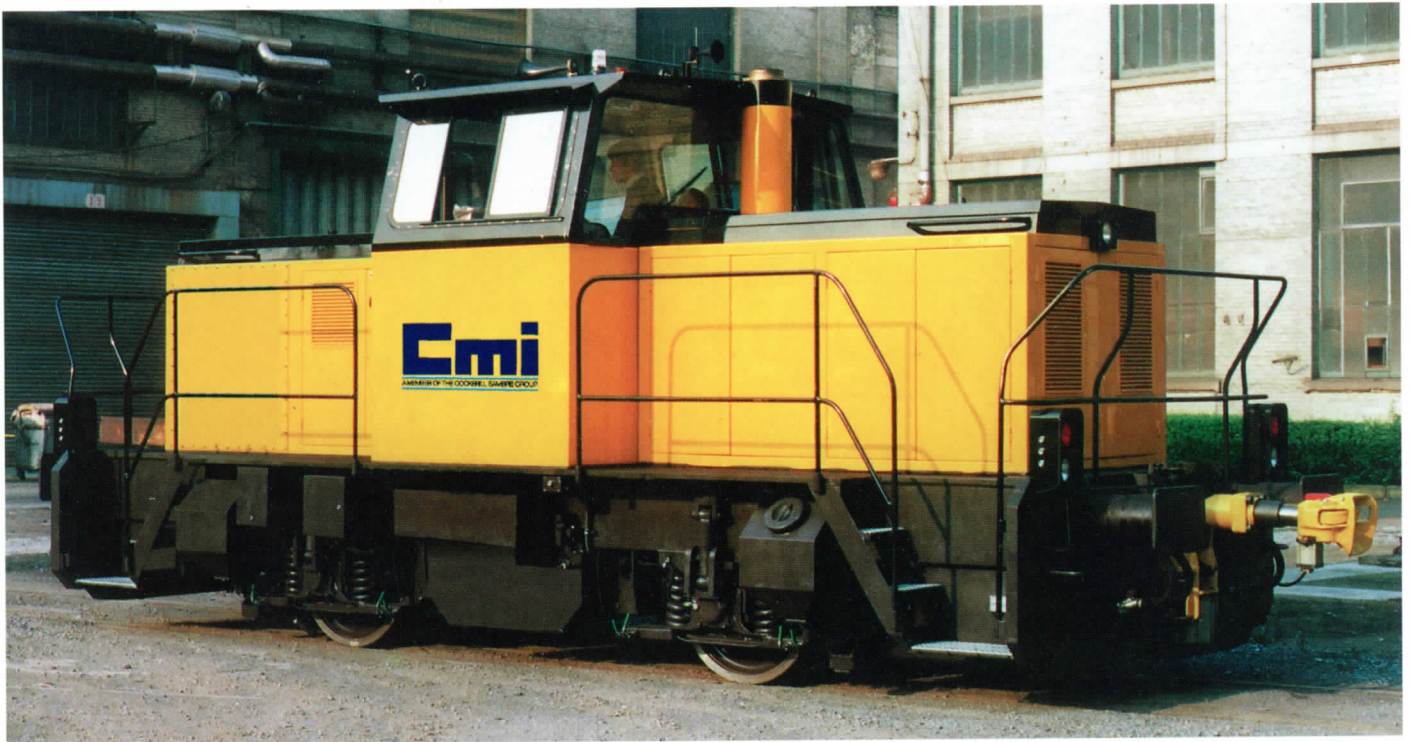
▲ The CMI hydrostatic shunting locomotive 525 HP
